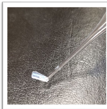
Fig. 1: homemade mini spatula for fishing out sections. Use a thin walled Eppendorf and carve out a slightly curved section into a fingernail shaped piece. Then heat up a Pasteur pipette, flatten the end to a 120 degree tilt, and then press into the plastic bit and hold until cool and bonded.
